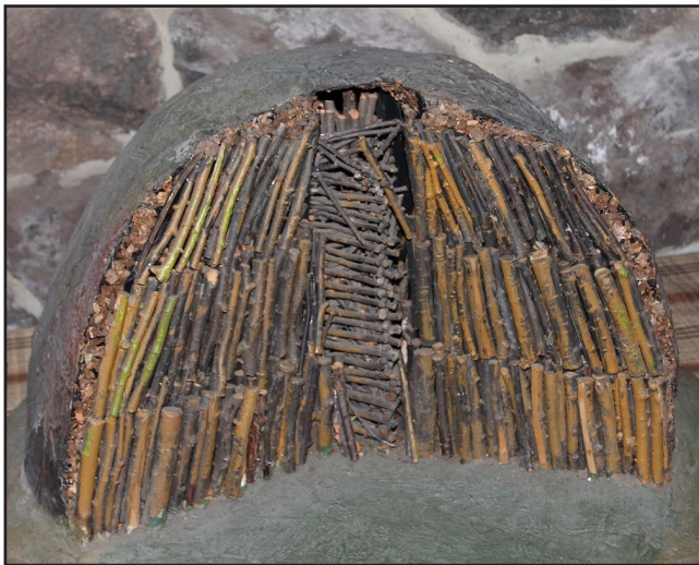
A three-tier charcoal pit. Notice the earthen covering on a layer of hardwood leaves (instead of pine needles) and a chimney in the center instead of lightwood. Photo courtesy of Douglas H. Page Jr.
